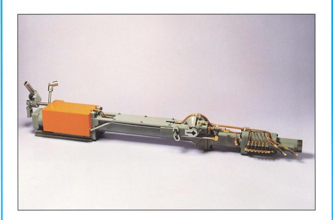
**Maul Technology** manufactures a complete range of Constant Cushion Take Out mechanisms to suit all IS. machine sizes. This rugged, well proven mechanism can be supplied with optional stabilisers and configured for overhead lubrication and cushion oil supply is maintained at a constant level and pressure by the independant oil system and provides smooth, repeatable deceleration at the end of each stroke.
